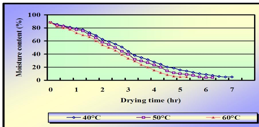
Fig. 1. Drying curves of solar dried roselle calyces.
