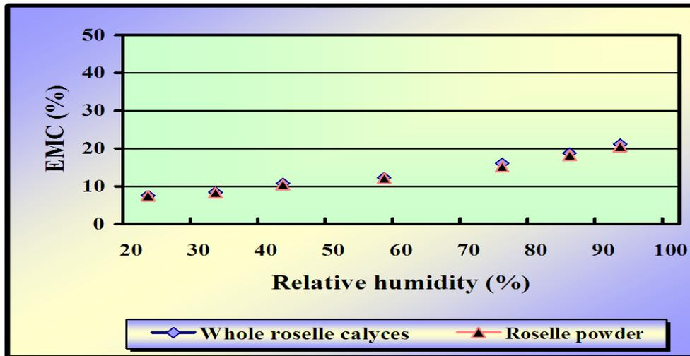
Fig. 3. Sorption isotherm curves of solar dried roselle samples (packaged in LDPE bags).
