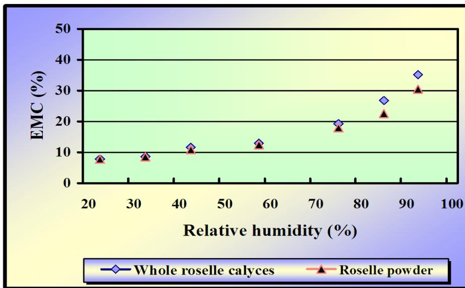
Fig. 2. Sorption isotherm curves of solar dried roselle samples (Without packaging).
