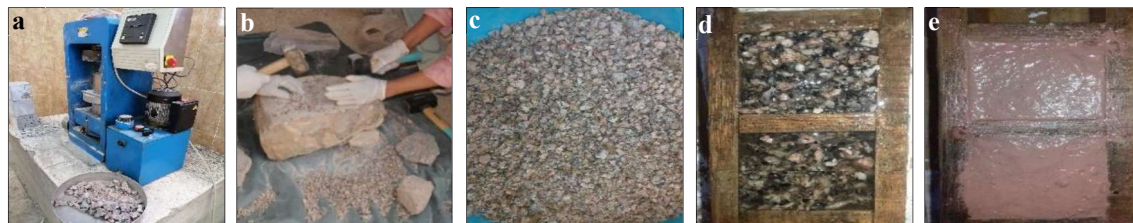
Figure (2) Shows a. & b. crushing granite by mac-hine and manually to obtain the required gain size, c. crushed granite, d. & e. preparation of cubes via pouring in a wooden mold lined with polyethylene sheets (5 cm×5 cm×5 cm)
