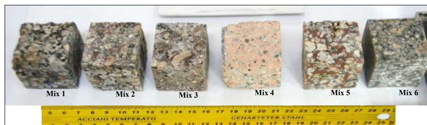
Figure (3) Shows examples of produced cubes of mixtures with dimensions of 5 cm×5 cm×5 cm
