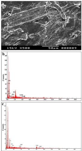
Figure (5) Shows <u>a</u>. SEM photo of the historical tracing paper sample, <u>b</u>. EDX analysis of the historical paper sample, <u>c</u>. EDX analysis of blue color
