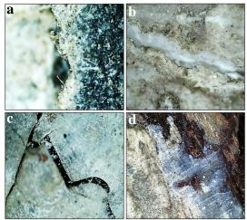
Figure (5) Shows USB digital microscope images deterioration aspects in the lower part of the mihrab, <u>a</u>. crusts at marble surface, <u>b</u>. dust and cracks in white marble units, <u>c</u>. salts under the surface layers of marble and flecking surface layer, <u>d</u>. wax used in the completion.
