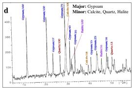
Figure (6) Shows XRD pattern, <u>a</u>. marble sample, <u>b</u>., salt sample from the bottom of the right column of the mihrab <u>c</u>. sample of the completion mortar used in a previous restoration on the top of the left column of the mihrab, <u>d</u>. sample of the mortar used to complement marble.
