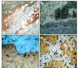
Figure (4) Shows USB digital microscope images of the top of the mihrab, <u>a</u>. dirt and dust in white and red marble units, <u>b</u>. complete the black marble by wax, <u>c</u>. micro-cracks and flake of the glaze layer of ceramic units, <u>d</u>. salts crystals and color stains on the ceramic body,
