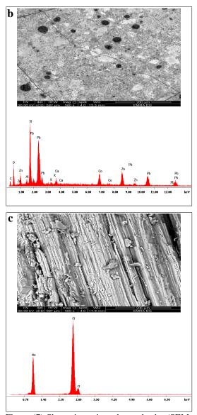
Figure (7) Shows investigated samples by (SEM-EDX), <u>a</u>. micrograph of calcite crystals and salt crystals (1000×), and EDX spectrum of marble, <u>b</u>. SEM micrograph of micro-cracks in the glaze layer, with the appearance of lead element (500×), and EDX spectrum of the same layer, <u>c</u>. SEM micrograph of sodium chloride (halite) (500×), and EDX spectrum of the sample of the salt from the mihrab
