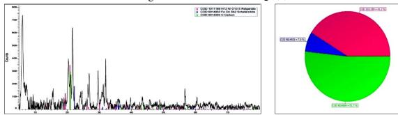
Figure (2) Shows X-ray patterns of the damaged components on the archaeological candle stand
