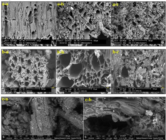
Figure (1) Shows SEM photomicrographs of (Sample 1); the bare wooden samples; <u>a-a</u>. erosion of cells notably vessels, <u>a-b</u>. & <u>a-c</u>. the consumption that took place in wood structure. (Sample 2); the bare wooden samples <u>b-a</u>. losing parts of the wood structure, <u>b-b</u>. & <u>b-c</u>. erosion of the cells due to beetles. (Sample 3); <u>c-a</u>. & <u>c-b</u>. the bare wooden samples structure deformation and the total collapse of wood
