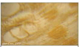
Figure (12) Fig. (12) OM photo of (T.S) section confirming that the type of the wood is Pinus nigra
