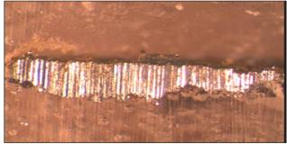
Figure (6) stereo-microscope photo the corrosion layers and the iron core of Hassan Pasha caravansary under.
