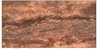
Figure (14) corrosion layers of Hassan Pasha caravansary under stereo-microscope.
