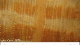
Figure (4) light microscope photo of (T.S) section confirming that the type of the wood is *Pinus sylvestris*
