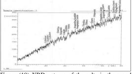
Figure (10) XRD paterns of the salts in the wood sample of Hassan Paha caravansary
