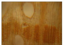
Figure (3) light microscope photo of (T.S) section confirming that the type of the wood is *Pinus nigra* (after, Core, H, 1979)
