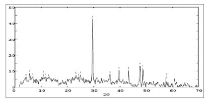
Figure (8) XRD pattern of plaster and colors as follow (Calcite CaCO<sub>3</sub>) (Hematite Fe<sub>2</sub>O<sub>3</sub>) **3.6. FTIR analysis**
