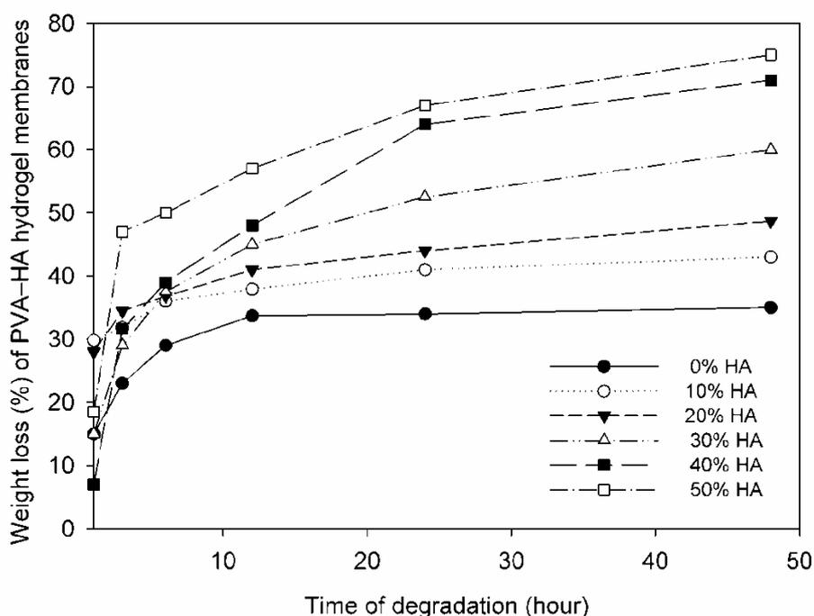
**Fig. 4-** Effect of HA contents on weight loss of the PVA-HA hydrogel membranes after different degrading times in phosphate buffer saline (PBS) (0.1 M, pH 7.4, at 37 °C).
