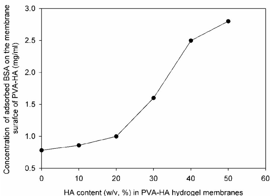
**Fig. 3-** Effect of Hyaluronic acid content on protein adsorption of PVA Hydrogel Membrane.
