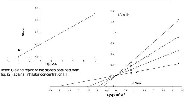
**Figure (2):** Competitive inhibition obtained from Lineweaver-Burk plot of 1/V versus 1/S, under the effect of alternariol on the rate of deamination of 5 HT by frontal cortex (MAO)extract (•) Control, ( $\Box$ ) 5.0, ( $\triangle$ ) 10.0 &(o) 15mmol/L.
