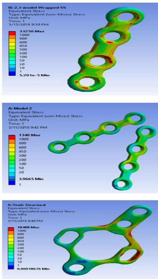
Fig. 3: Von Misses stresses for Titanium plates
