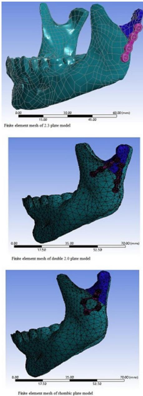
Fig. 1: Finite element mesh of the three different models
