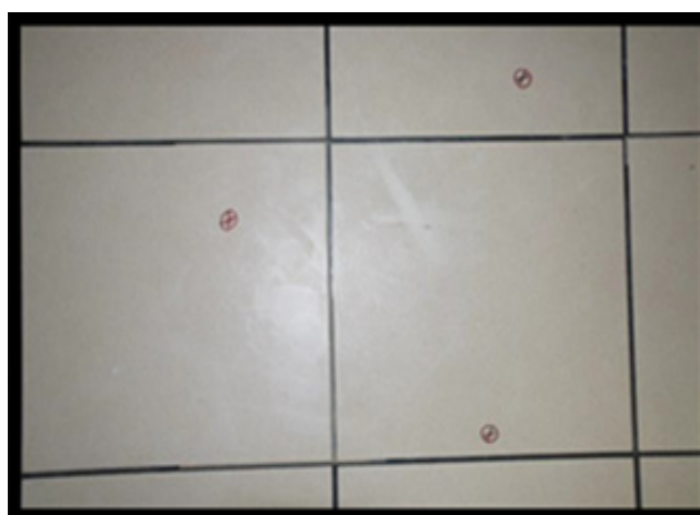
Fig. 4: Three permanent markers on the floor to accurate positioning of the tripod legs every time.
