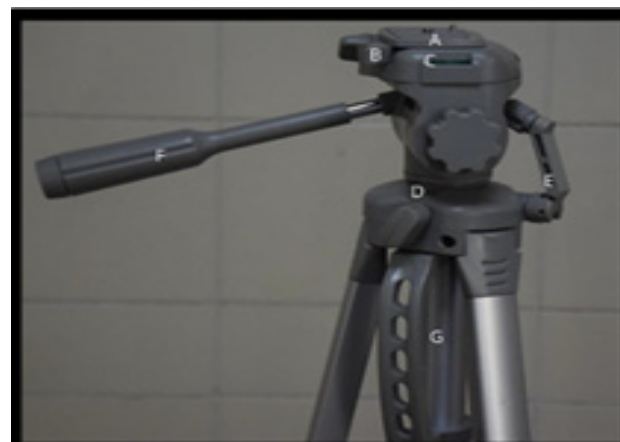
Fig. 5: Tripod Components (Walimex WT-3570 Basic Tripod). A) Quick releasing plate. B) Quick releasing mount plate. C) Horizontal spirit level. D) Round spirit level. E) Crank handle. F) Pan handle. G) Housing of Central column.
