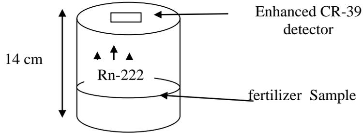
**Figure (3):** A schematic diagram of the sealed –cup technique in fertilizer sample.
