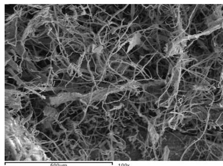
**Fig. 1:** FT-IR for rice straw-pulp**Fig. 2:** SEM for rice straw –pulp
