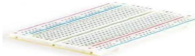
Figure. 5: The breadboard.
