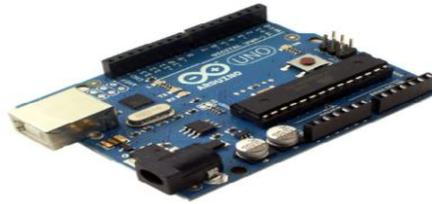
Figure. 1: The Arduino Uno.
