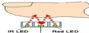
Figure. 6: The MAX30102 sensor.
