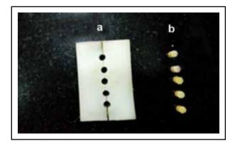
Fig. (1) (a): Teflon split molds used for preparation of compressive strength samples Fig. (1) (b): Prepared samples.
