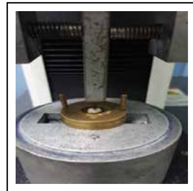
Fig. (1) Sample during push out test
