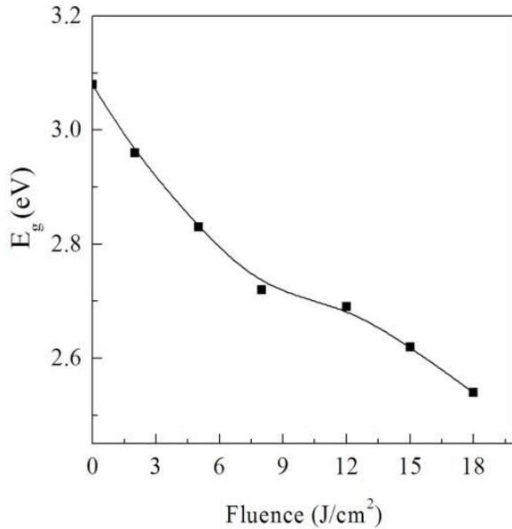
**Fig. (4): The change of optical band gap  $E_g$  with the laser fluence**
