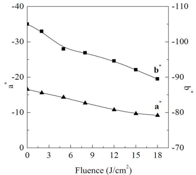
Fig. (9): The change of  $a^*$  and  $b^*$  color intercepts with the laser fluence
