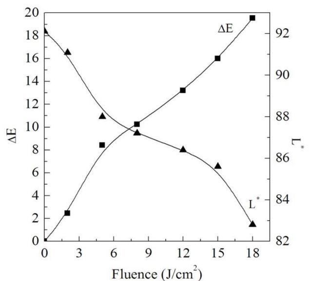
Fig. (10): The change of  $L^*$  color intercept and color intensity  $\Delta E$  with the laser fluence
