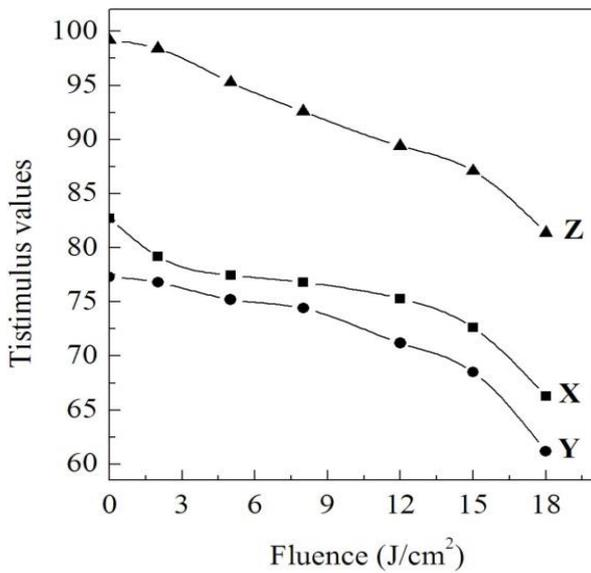
Fig. (7): The change of tristimulus values with the laser fluence
