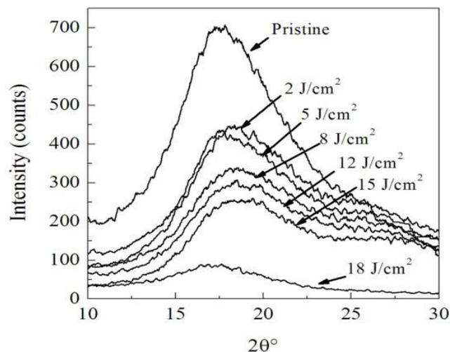
Fig. (1): XRD patterns of the Mak samples
