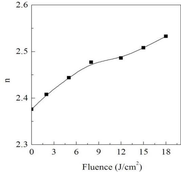
**Fig. (5): The change of refractive index with the laser fluence**
