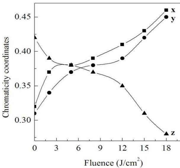
Fig. (8): The change of chromaticity coordinates with the laser fluence
