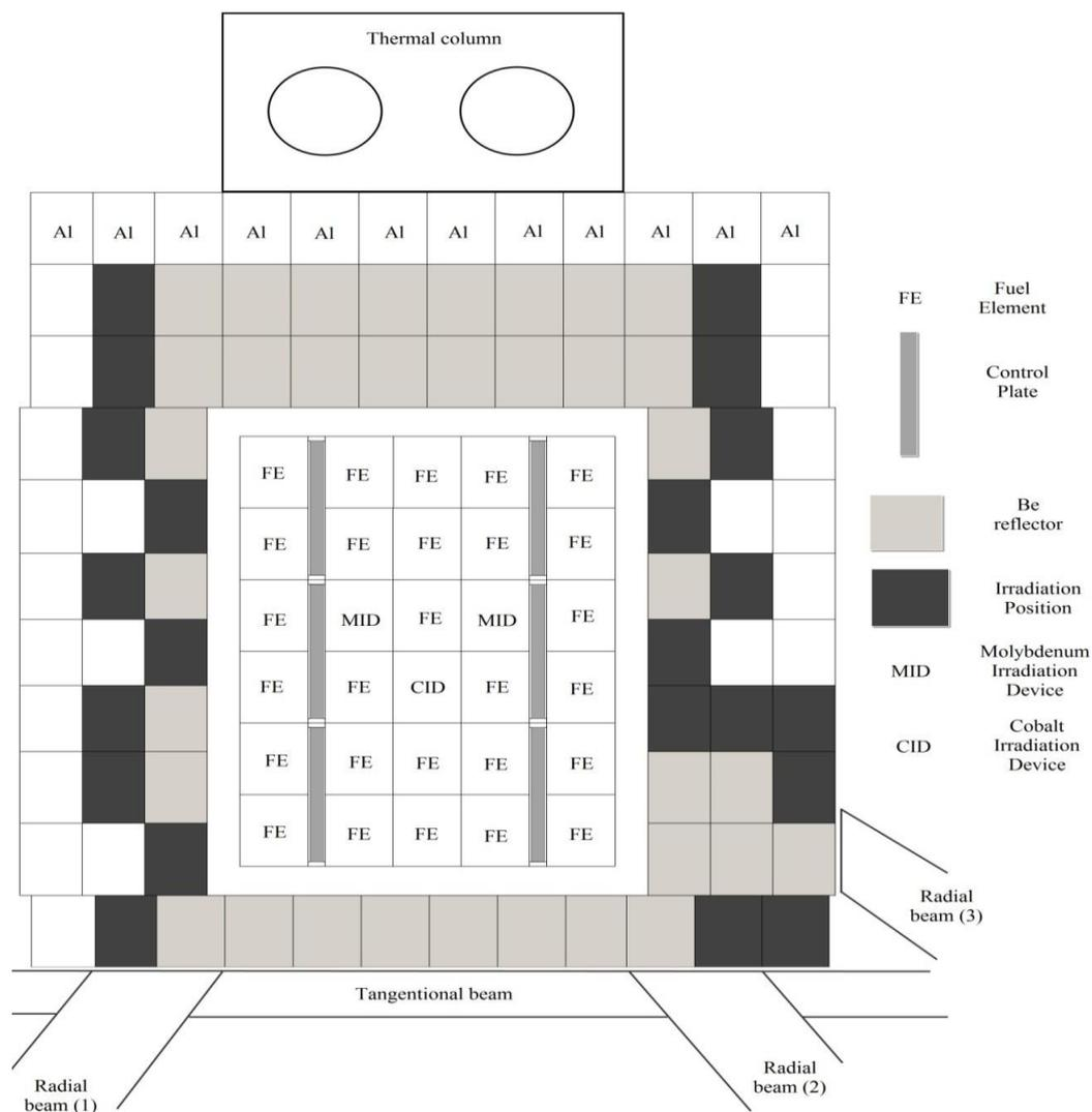
Fig. (1): ETRR-2 core and beam tube
