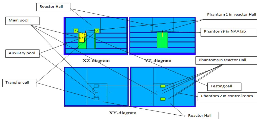
Fig. (4): the phantoms in the reactor building in different distributions
