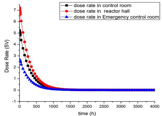
**Fig. (6): External photon dose rate decay in three positions for a  $I^{131}$  gas cloud dispersed throughout the reactor hall with time**
