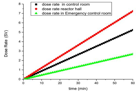
**Fig. (5): External photon dose rate to phantoms in three positions for a  $I^{131}$  gas cloud with time**
