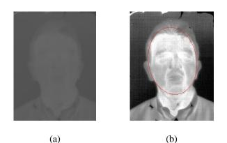
Fig. (1): The steps of direct least ellipse fitting algorithm face detection. (a) original Infrared Image, (b) face detected region with the ellipse fitting algorithm
