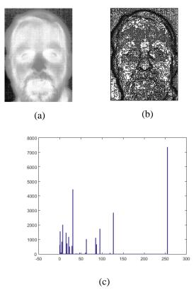
Fig. (2): show the step of LBP (a) Infrared image, (b) LBP image and (c) LBP Histogram of image
