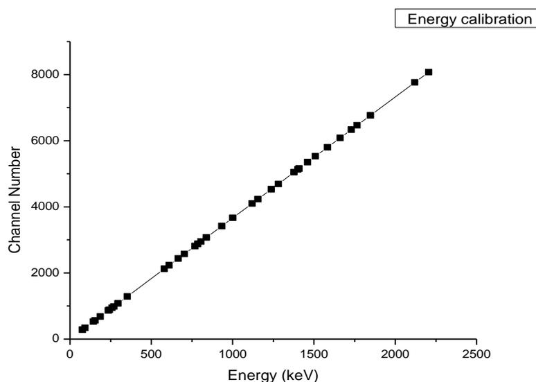
Fig. (1): Energy calibration for high purity germanium detector
