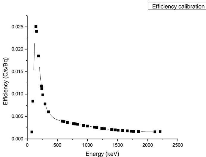
**Fig.(2): Efficiency calibration for high purity germanium detector**
