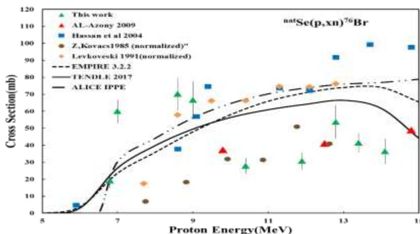
Fig. (1): Excitation function for  $^{nat}\text{Se}(p,xn)^{76}\text{Br}$
