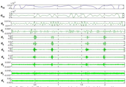
Fig. (7): Wavelet Coefficients for normal sound signal at tenth level of decomposition
