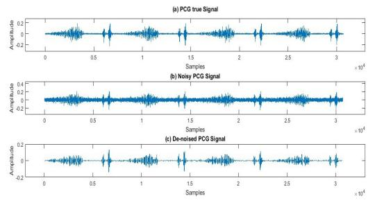
Fig. (3): Denoising of PCG acoustic signal using Db10 wavelet with fourth level and hard thresholding
