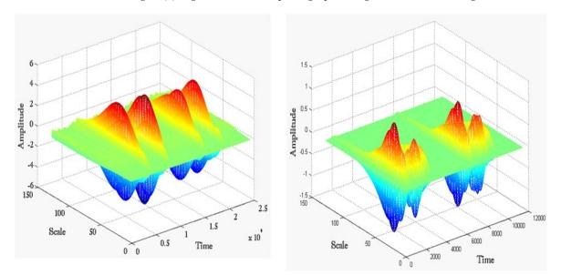
Fig. (5): Spectral information of normal PCG acoustic signal using WT (a) High Resolution 2D spectrographic image of Normal PCG signal (b) High Resolution 2D spectrographic image of abnormal PCG signal
