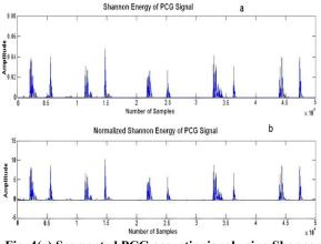
Fig. 4(a) Segmented PCG acoustic signal using Shannon energy (b) Normalized Shannon energy for PCG signals
