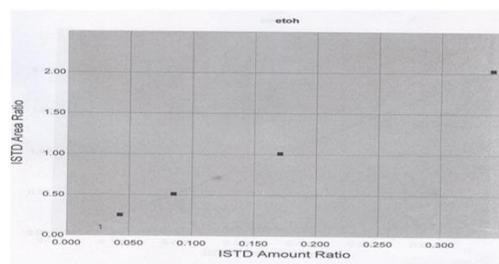
Figure 2: Linearity of Calibration curve for ethanol using GC-HS
