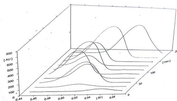
Figure 5: HPTLC Chromatogram of all tracks including sample and standard at 254 nm  $\lambda$  max
