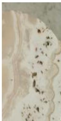
**Figs.144-147** Display the form of small pits - are caused by biogenically induced corrosion processes, particularly in carbonate rocks , it is noticed only on the Egyptian alabaster surfaces of Muhammad Ali Mosque , it is not noticed on the surfaces of chapels at Karnak
