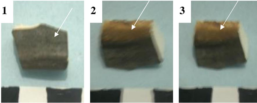
**Fig. 117** Dark ( grey - to black colored crust of compact deposits on the surface of a part of an Egyptian alabaster of Muhammad Ali Mosque changing the surface in (1) (arrow) , partially changing the surface and partially tracing the surface in (2) (arrow) and tracing the surface in (3) (arrow) , so it is of compact deposit of pollutants of the atmosphere mainly of gypsum crust including dirt .
