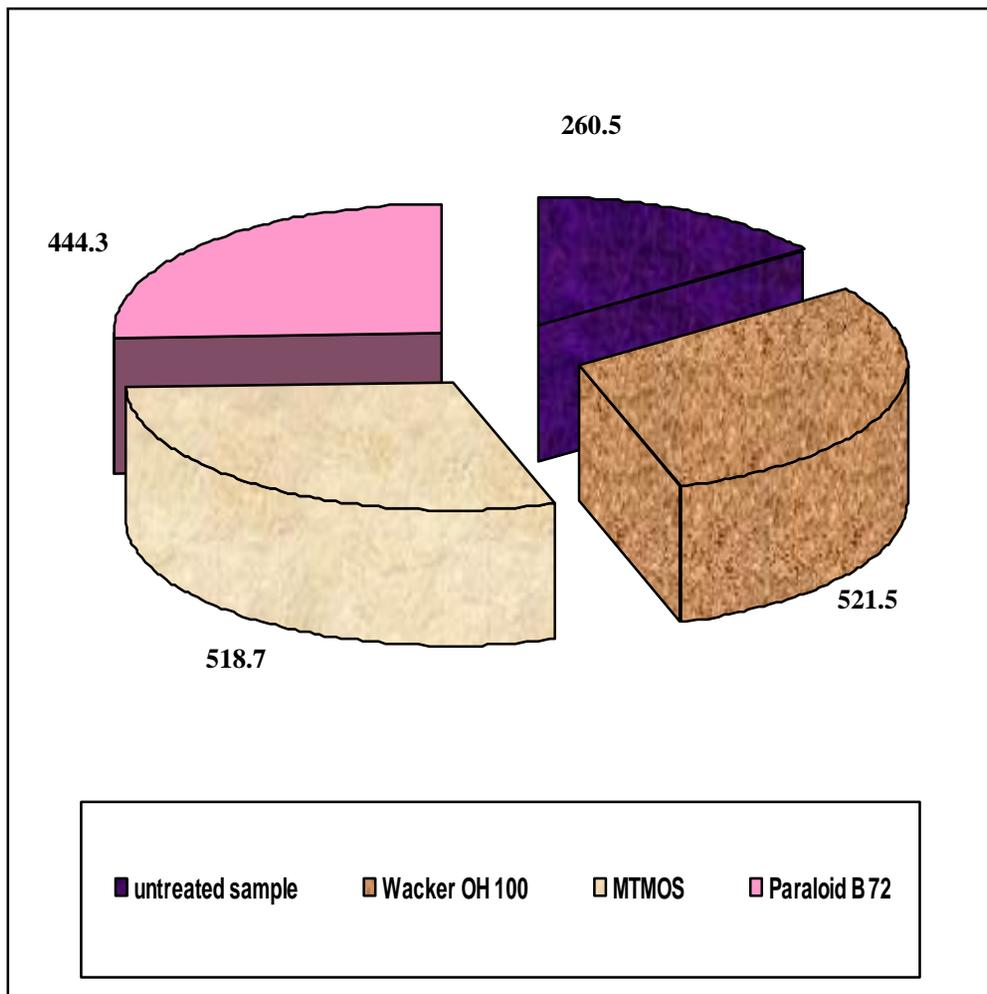
**Fig.175** display the Improvement of Egyptian alabaster weathered Karnak chapels of samples of compressive of strength (wet) from (260.5) in untreated sample to (444.3) with Paraloid B 72 , to (518.7) with MTMOS and to (521.5) with Wacker OH 100.
