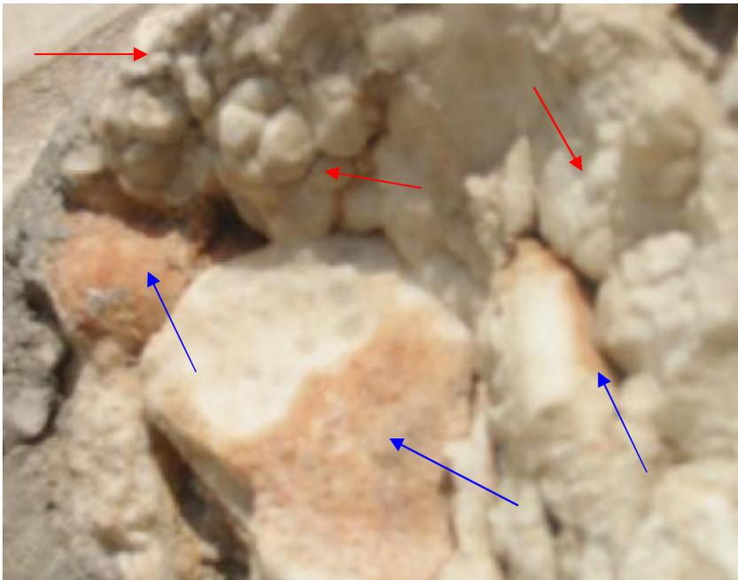
**Figs.96-97** Display the iron oxides inside the Egyptian alabaster in both Karnak (left) and Muhammad Ali Mosque veneers(right) (blue arrows) which existed as impurities and which are not responsible the coloration of the Egyptian alabaster, also the granular disintegration into grus can be observed in lower photo (red arrows).
