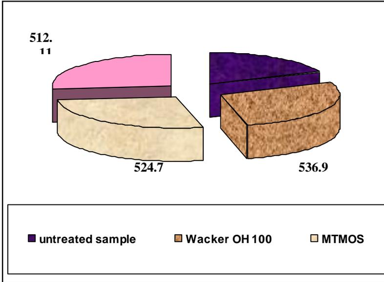
**Fig.170** display the Improvement of Egyptian alabaster weathered samples of Muhammad Ali Mosque veneers of compressive of strength (dry) from (375.5) in untreated sample to (512.1) with Paraloid B 72 , to (524.7) with MTMOS and to (524.7) with Wacker OH 100.
