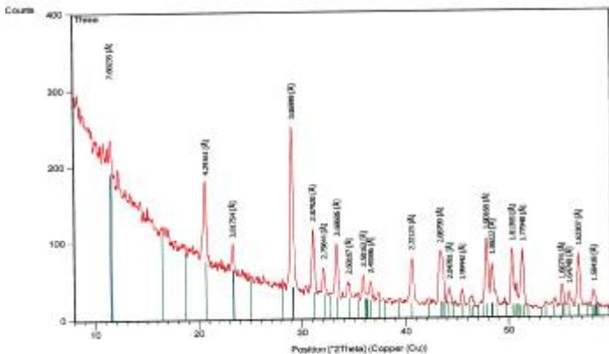
Figs . 118-119 X-ray diffraction pattern of Dark ( grey - to black colored) crust of compact deposits on the surface of a part of an Egyptian alabaster of Muhammad Ali Mosque , exhibits the presence of Gypsum  $CaSO_4 \cdot 2H_2O$  and  $Ca(SO_4)(H_2O)_2$  , due to atmospheric pollution , the continental climate , air dust , wet, porous, sheltered and semi-sheltered surfaces
