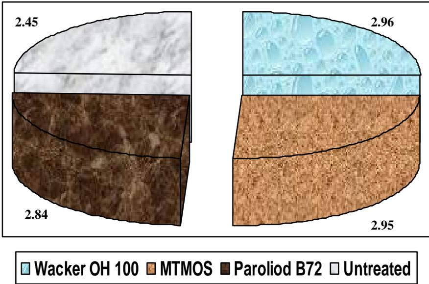
**Fig. 172** display the Improvement of weathered samples of Egyptian alabaster of Karnak chapels of Bulk density from (2.45) in untreated sample to (2.84) with Paroliod B 72 , to (2.96) with Wacker OH 100 and to (2.95) with MTMOS .
