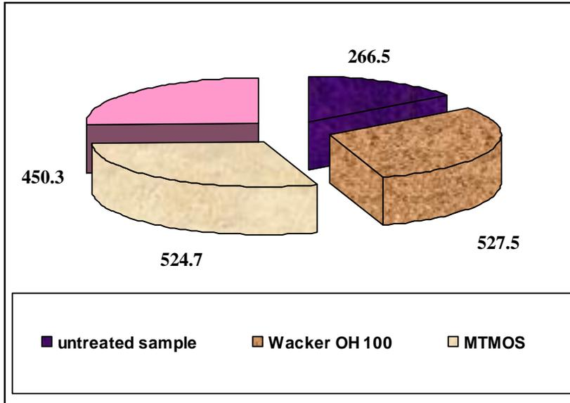
**Fig.171** display the Improvement of Egyptian alabaster weathered samples of Muhammad Ali Mosque veneers of compressive of strength (wet) from (266.5) in untreated sample to (450.3) with Paraloid B 72 , to (524.7) with MTMOS and to (527.5) with Wacker OH 100.
