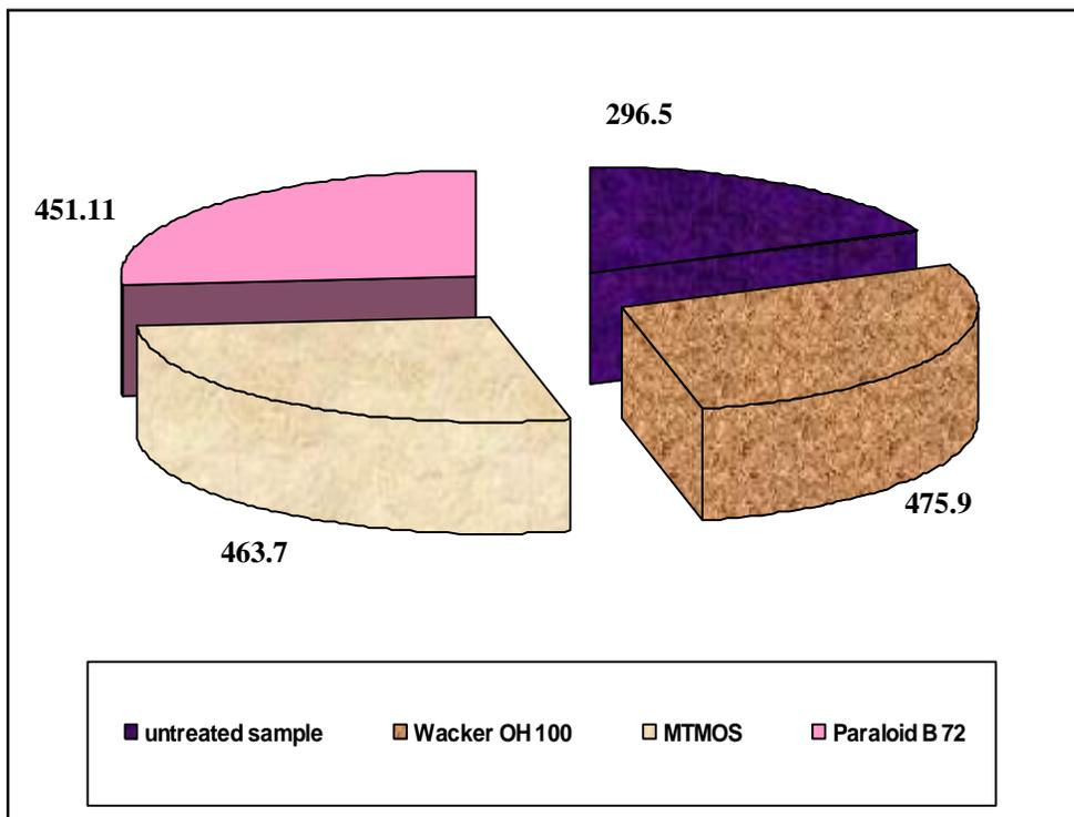
**Fig. 174** display the Improvement of Egyptian alabaster weathered samples of Karnak chapels of compressive of strength (dry) from (296.5) in untreated sample to (451.11) with Paraloid B 72 , to (463.7) with MTMOS and to (475.9) with Wacker OH 100.
