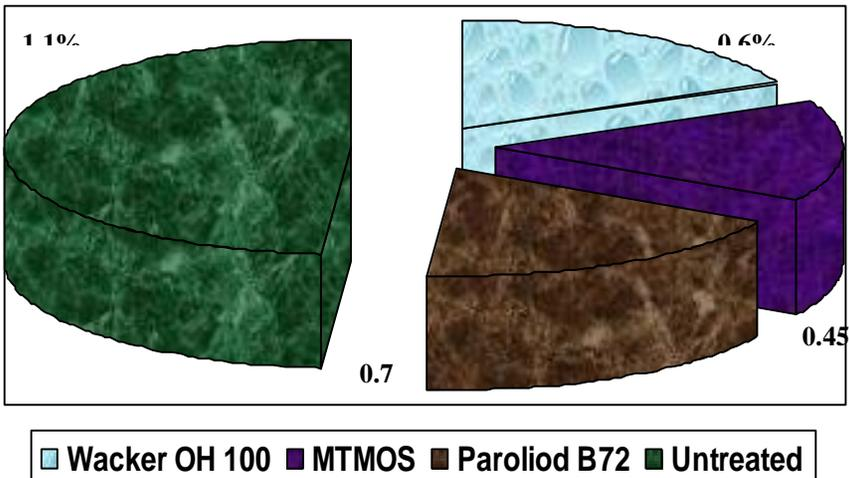
**Fig.173** display the Improvement (reduction) of Egyptian alabaster weathered samples of Karnak chapels of Water absorption from (1.1 %) in untreated sample to (0.7 %) with Paroliod B 72 , and to (0.45 %) with MTMOS , and to (0.6 %) with Wacker OH 100..
