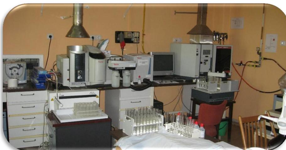
Atomic absorption for measuring the content of elements in soil, plant and water samples
