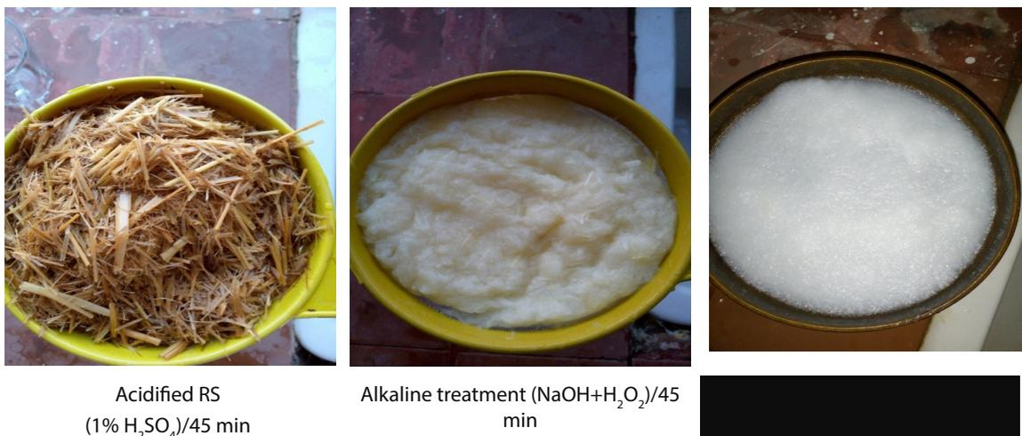
Fig. 1. The preparation steps of the sorbent
