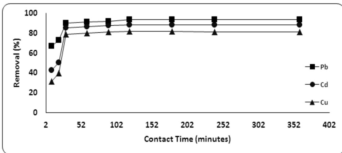
Fig. 7. Effect of contact time (minutes) on the removal of the PTEs (Pb, Cd, and Cu) from their aqueous Solutions by MCC
