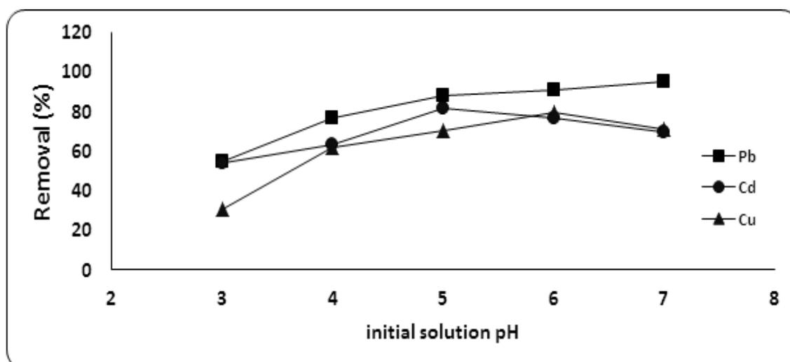
**Fig. 6. Effect of pH of solution on removal of the PTEs Pb, Cd, and Cu from their aqueous solutions using Microcrystalline cellulose MCC**
