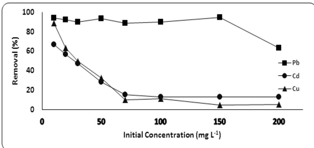
Fig. 5. Effect of solution initial metal ion concentration ( $\text{mg L}^{-1}$ ) on removal of the PTEs lead, Cadmium and Copper from their aqueous solutions using Microcrystalline cellulose MCC.
