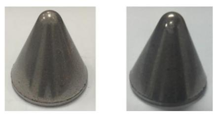
Fig. 4: A pressed (left) and sintered (right) PTFE/W/Cu/Pb SC liner.
