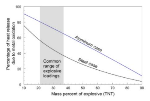
Fig. 2: Estimation of the contribution of the heat released if complete oxidation of a metal case occurs for a munition containing 30% TNT as explosive<sup>[2]</sup>.
