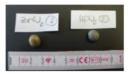
Fig. 6: Two samples of approximately 5 g of ZrW2 and HfW2. ZrW2 has a more "golden" color, whereas HfW2 is silvery-metallic.
