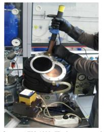
**Fig. 5:** Arc-furnace AF92-1000. The long copper electrode can be moved up and down and turned around by a circle-movement. Between the electrode and the outer casing of the arc-furnace there is a tension of about 15 V, therefore, the operator uses isolating gloves.
