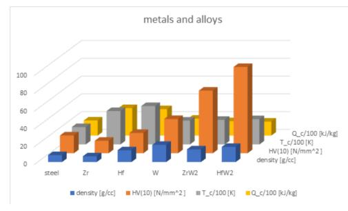
Fig. 6: Selected properties of metals and alloys
