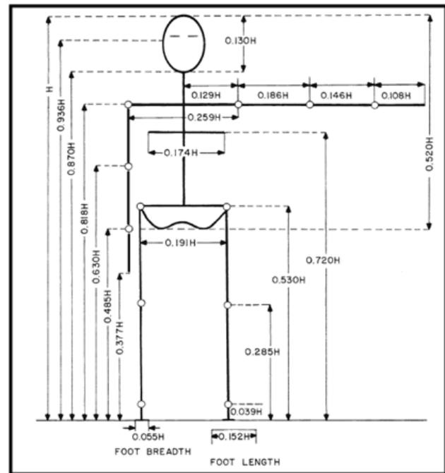
Fig. 2: Dimensions of body segments relative to height<sup>[16]</sup>.
