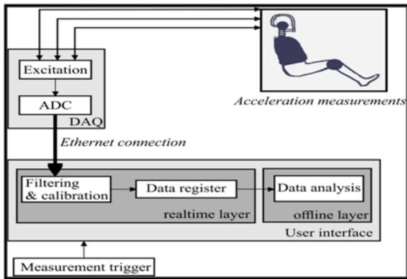
Fig. 9: A schematic of the measurement system connections
