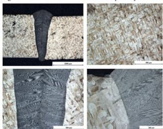
**Fig. 4:** Microstructure of laser welding of sample L1. (a) Overview with 2000 $\mu$ m scale bar, (b) base material with 500 $\mu$ m scale bar, (c) weld region with 500 $\mu$ m scale bar and (d) weld and HAZ with 200 $\mu$ m scale bar.
