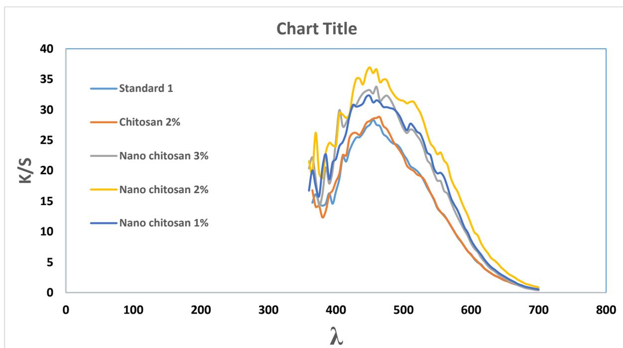
Fig. 1. Effect of wavelength on K/S for wool dyed with direct dye by Conventional method
