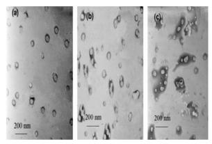
Figure 6. TEM images of Acrylic–polyurethane hybrid emulsion with polyacrylic/polyurethane ratios of (a) 40/60 (PUA 40), (b) 60/40 (PUA 60) and (c) 80/20 (PUA 80)
