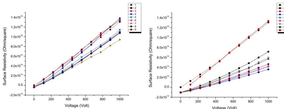
**Fig. 2:** Surface resistivity of untreated (left) and bio-treated (right) knitted PET/L blended fabrics with different blending ratios
