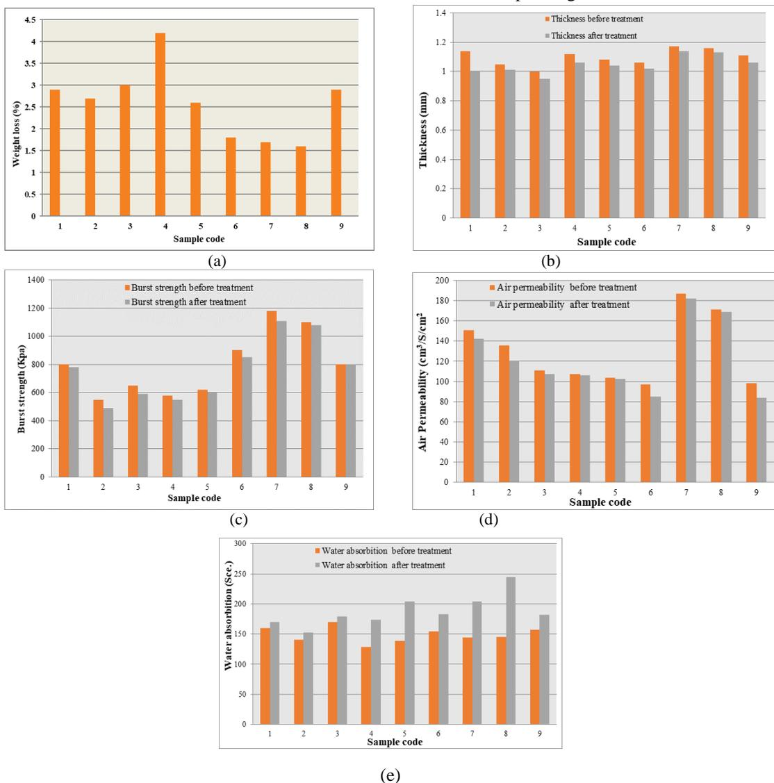
**Figure1 (a-e):** Effect of bio-treatment of with PET/L fabrics of different blending ratios on their wight (a), thickness (b), burst (c), air permeability (d), and water absorption (e)
