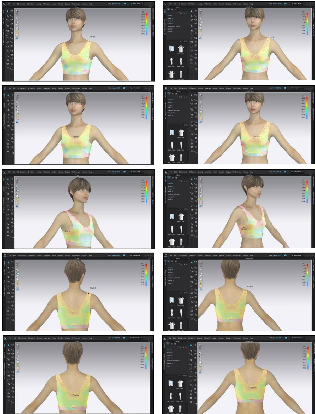
**Figure 4:** CLO3D Simulation System for evaluation of fitting and stretch-ability of sample number 7 (light weight 92/8 knitted PET/L blended fabric)
