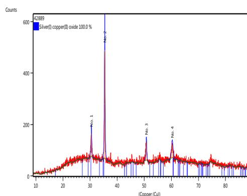
Fig. 2: XRD patterns of 5% Ag/CuO nanoparticle thin film on silicon.
