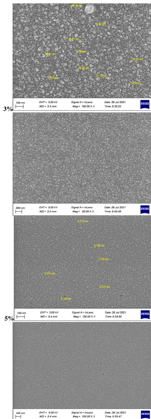
Fig.7: FESEM images of Ag/CuO thin-film Si sample.
