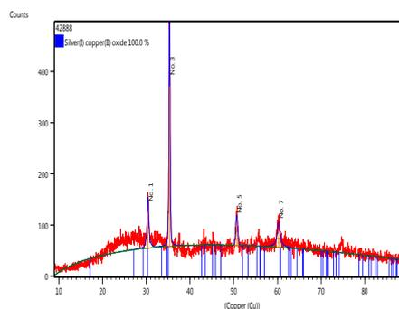
Fig. 1: XRD patterns of 3% Ag/CuO nanoparticle thin film on silicon.
