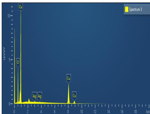
Fig.5: EDX spectrum of 3%Ag/CuO nanoparticles sample.
