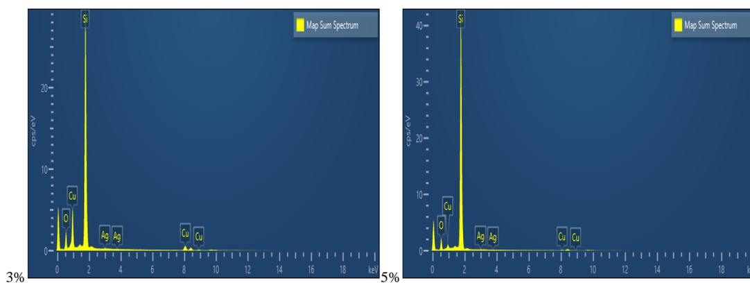
Fig.9: EDX spectra of Ag/CuO deposited on Si
