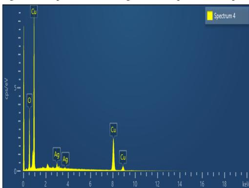
Fig.6: EDX spectrum of 3%Ag/CuO nanoparticles sample.
