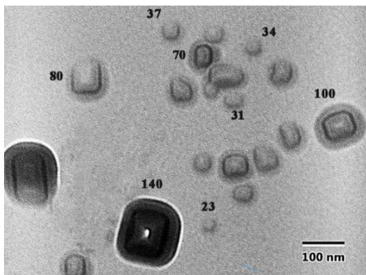
Fig.3. TEM image of *C. crinita*-mediated synthesized ZnO-NPs.
