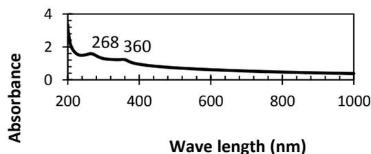
Fig.2. UV-Vis spectrum of ZnO-NPs synthesized by *C. crinita*.
