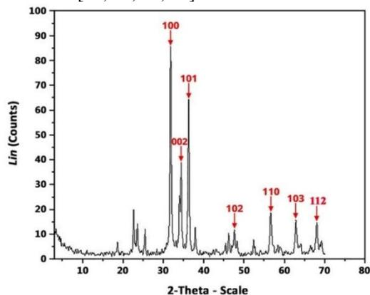
Fig. (4): XRD patterns of *C. crinita*-mediated synthesized ZnO-NPs.
