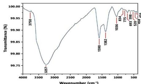
Fig. 5. FTIR spectrum of *C. crinita*-mediated synthesized ZnO-NPs.
