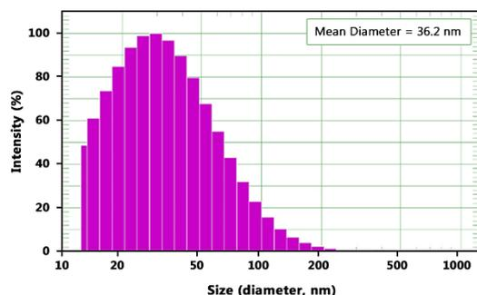
**Fig. 7.** DLS graph of *C. crinita*-mediated synthesized ZnO-NPs.
