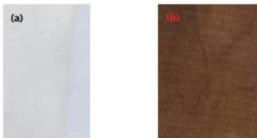
**Fig. 2 :Photographic image of (a) untreated nylon fabric (b) biosynthesized CuNPs nylon fabric .**
