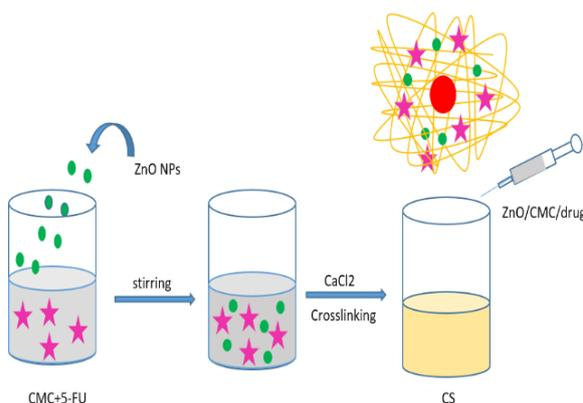
Graph (1): Preparation of ZnO-CMC-CaCl<sub>2</sub>/CS hybrids by ionotropic gelation
