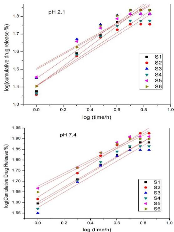
Figure (7): kinetic release of 5-FU from samples S1-S6 according to Korsmeyer-Peppas model at pH 2.1 and pH 7.4.
