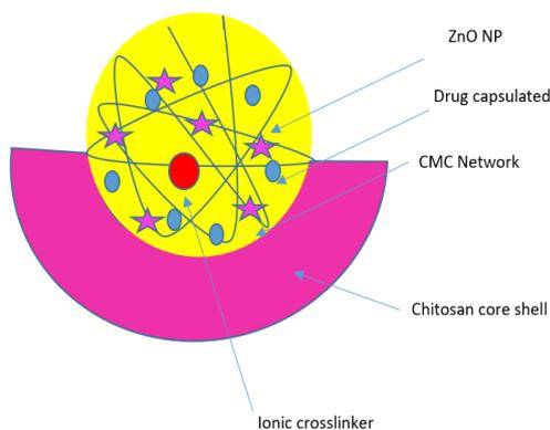
Graph (2): Schematic representation of the self-assembly cross-linking
