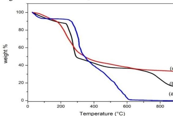
Figure (2): TGA of a) native chitosan, b) native Na-CMC and c) CS/ZnO-CMC/CaCl<sub>2</sub>
