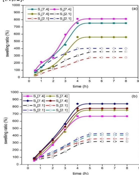
Figure (5): Swelling behavior of CS/ZnO-CMC/CaCl<sub>2</sub> samples at pH 2.1 and 7.4 (a) Effect of polymer content for samples S1-S3, and (b) Effect of ZnO NPs content for samples S1 and S4-S6.
