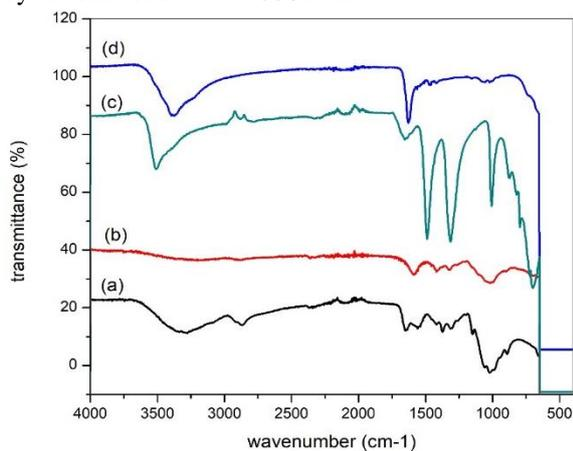
Figure (1): FTIR spectrum for (a) pristine chitosan, (b) pristine CMC and (c) CS/ZnO-CMC/CaCl<sub>2</sub>
