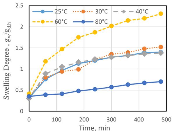
Figure (2) Swelling Degree in Terms of Water Absorbed Per Dry Hydrogel as a Function of Time
