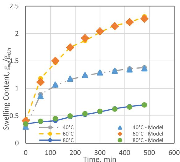
Figure (5) Comparison between model predictions and experimental results at 40, 60, and 80°C
