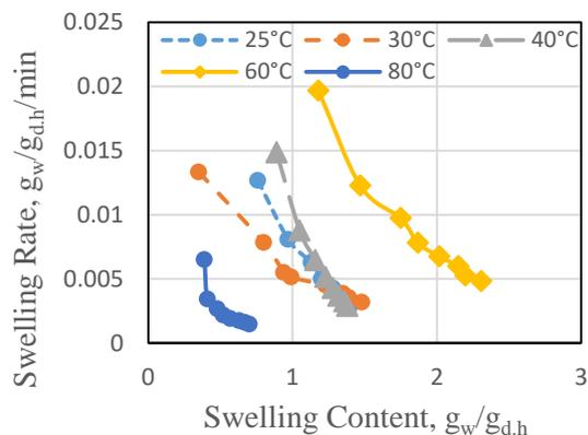
Figure (6): Relation Between the Swelling Rate and The Swelling Degree at Different Temperatures
