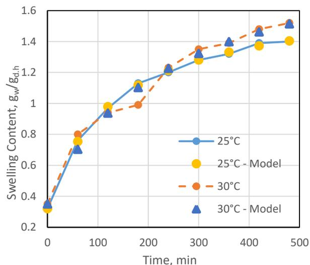
Figure (4) Comparison between model predictions and experimental results at 25 and 30°C
