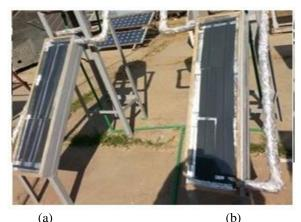
Figure 4 Set up of a prototype of solar water heating system. (a) Prepared of black colored nano porous anodized aluminum, (b) matte black paint absorber
