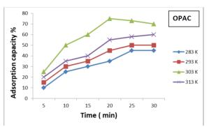
Fig. 8 . Effect of temperature on adsorption capacity by OPAC
