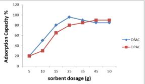
Fig. 5. Effect of sorbent dosage on adsorption capacity of OSAC and OPAC
