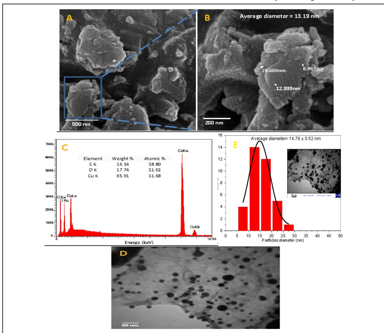
**Figure 2.** (A and B) FE-SEM images of CuO-NPs at different magnifications, (C) EDX spectrum of CuO-NPs. (Inset; Quantitative elemental analysis), (D) TEM for CuO-NPs, (E) particle size distribution histogram.
