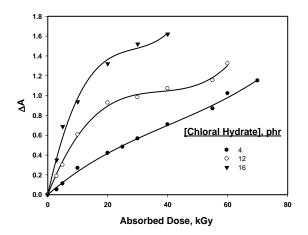
Fig 3. Change of  $\Delta A$ . of O IV/ IC/ PVA films containing different chloral hydrate concentrations. [O IV]= 0.32 phr, [IC] = 0.04 phr, at  $\lambda$ max= 448 nm.
