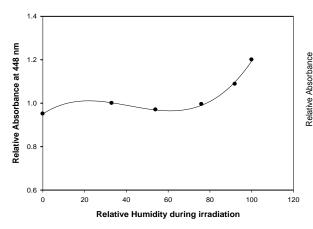
Fig. 4 Variation of response of O IV/ IC/PVA film as a function of relative humidity during irradiation 3.4 Pre-irradiation stability
