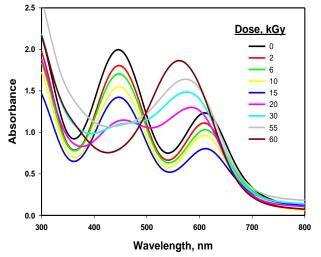
Fig 2: Absorption Spectra of unirradiated and irradiated O IV/ IC/ PVA film containing chloral hydrate at different absorbed dose.[ O IV= 0.32 phr], [ IC= 0.04 phr ], [ CH= 16 phr]
