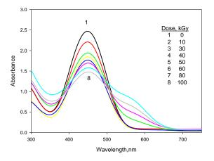
Fig.1a Absorption Spectra of unirradiated and irradiated O IV/PVA film containing chloral hydrate at different absorbed doses. [ O IV=0.32 phr ], [ CH= 8 phr ]
