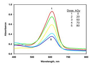
Fig.1b Absorption Spectra of unirradiated and irradiated IC/ PVA film containing chloral hydrate at different absorbed doses. [ IC= 0.04 phr ], [ CH= 16 phr ]
