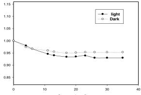
Storage time, Days Fig. 6. Post-irradiation stability of O IV/ IC/ PVA films stored in diurnal cycles of day light at room temperature in 25°C at 448 nm.
