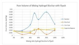
Fig 2: Pore volume of mixing hydrogel biochar
