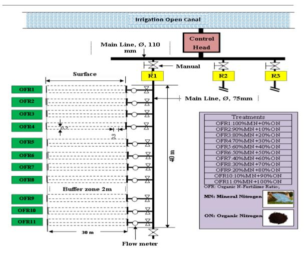
Figure (1): Layout of experimental design.
