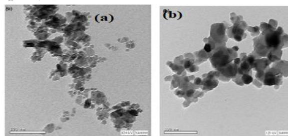
**Fig.5.**HR-TEM micrographs for  $\text{Cu}_x\text{Zn}_{(1-x)}\text{Al}_2\text{O}_4$  where a)  $x$  is 0.0, b)  $x$  is 1.0 molar ratios using co-precipitation method loaded with carbon spheres
