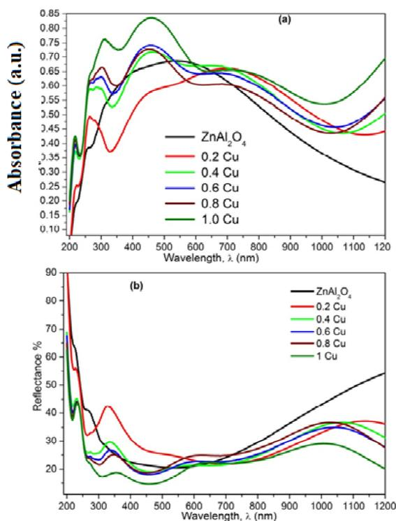
**Fig.8.** (a) Absorbance (b) Reflectance of  $\text{Cu}_x\text{Zn}_{(1-x)}\text{Al}_2\text{O}_4$  nano-powders (where  $x = 0.0, 0.2, 0.4, 0.6, 0.8, 1.0$ ), using co-precipitation method loaded with carbon spheres
