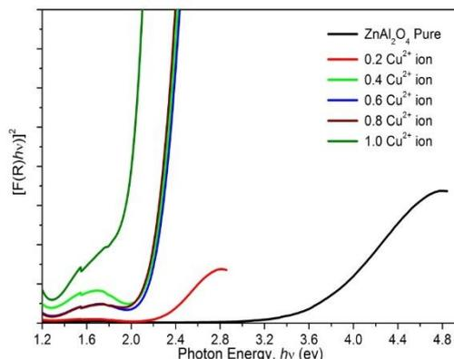
**Fig.7 Optical energy gap of  $\text{Cu}_x\text{Zn}_{(1-x)}\text{Al}_2\text{O}_4$  nano-powders (where  $x = 0.0$  to  $1.0$ ) by using co-precipitation method non-loaded with CSs**
