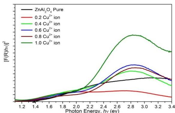
**Fig.9** Optical energy gap of  $\text{Cu}_x\text{Zn}_{(1-x)}\text{Al}_2\text{O}_4$  nano-powders( where  $x = 0.0$  to  $1.0$ ) using co-precipitation method loaded with carbon spheres
