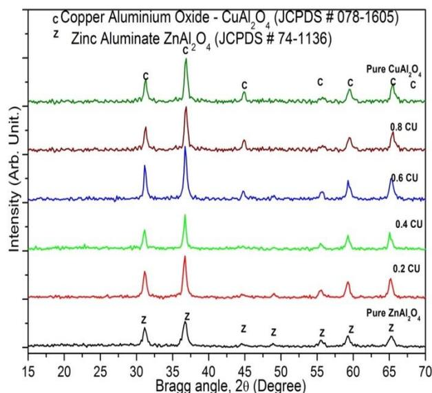
**Fig.2** XRD patterns of  $\text{Cu}_{(x)}\text{Zn}_{(1-x)}\text{Al}_2\text{O}_4$  ( $x$  from 0.0 to 1.0 molar ratios) using co-precipitation and loaded with carbon spheres
