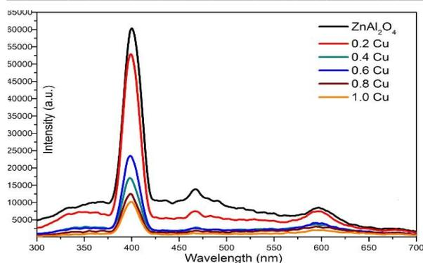
**Fig. 10** PL of  $\text{Cu}_{(x)}\text{Zn}_{(1-x)}\text{Al}_2\text{O}_4$ , nano-powders (where  $x = 0.0, 0.2, 0.4, 0.6, 0.8, 1.0$ ) by using co-precipitation method non-loaded with CSs
