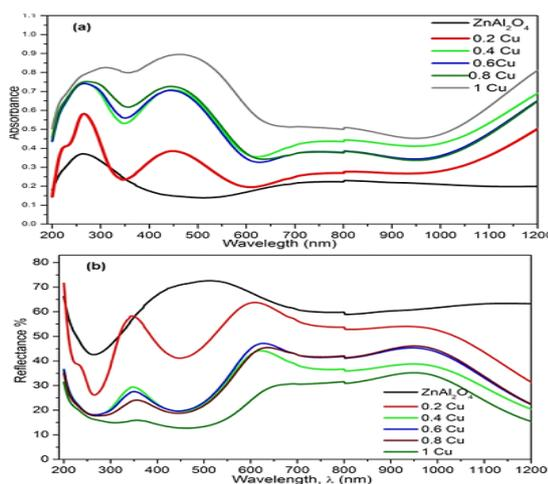
**Fig.6: (a) Absorbance (b) Reflectance of  $\text{Cu}_x\text{Zn}_{(1-x)}\text{Al}_2\text{O}_4$  nano-powders (where  $x = 0.0, 0.2, 0.4, 0.6,$**
