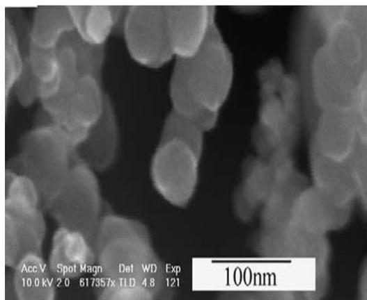
**Fig.3** FESEM micrographs of carbon sphere
