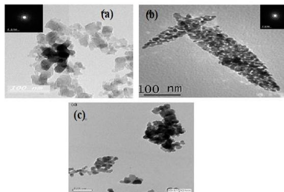
**Fig.4.**HR-TEM micrographs for  $\text{Cu}_x\text{Zn}_{(1-x)}\text{Al}_2\text{O}_4$  where a)  $x$  is 0.0, b)  $x$  is 0.6 molar ratios and c)  $x$  is 1.0 molar ratios annealed at  $1000^\circ\text{C}$  for 2 h using co-precipitation method not loaded with carbon spheres
