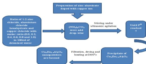
Scheme1: Synthesis of zinc aluminate doped with Cu (II) nanoparticles using co-precipitation method non-loaded with carbon spheres
