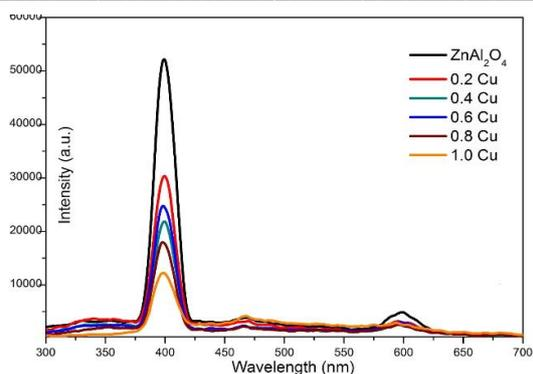
**Fig. 11.** PL of  $\text{Cu}_{(x)}\text{Zn}_{(1-x)}\text{Al}_2\text{O}_4$ , nano-powders (where  $x = 0.0, 0.2, 0.4, 0.6, 0.8, 1.0$ ) using co-precipitation method loaded with carbon spheres
