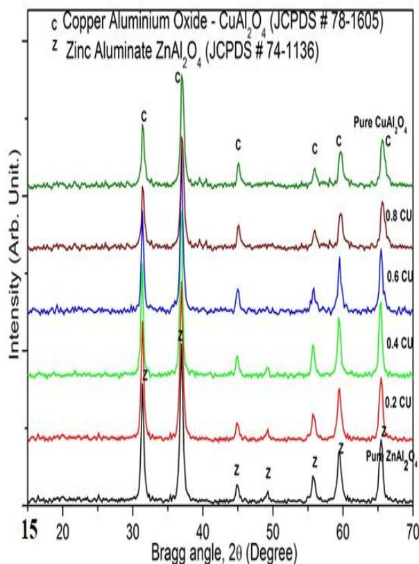
**Fig 1:** XRD patterns of  $Cu_{(x)}Zn_{(1-x)} Al_2O_4$  ( $x$  from 0.0 to 1.0 molar ratios) annealed at 1000 °C for 2 h using co-precipitation
