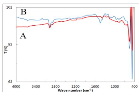
Fig. 3. (A, B) FTIR spectrum of ZnO nanoparticles (A) prepared without using TEA and (B) ZnO prepared with using Triethanolamine.
