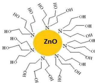
Fig. 1. A schematic representation of capped ZnO nanoparticles.
