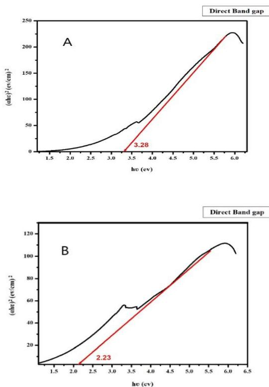
Fig. 9. The band gap for ZnO nanoparticles A and B.
