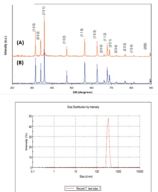
Fig. 2. (A, B). XRD pattern of the ZnO powders synthesized without using TEA (A) and using TEA (B).
