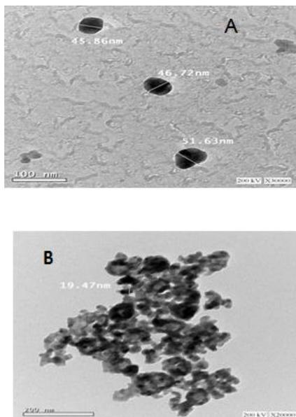
Fig. 6. (A, B) TEM images of ZnO powders synthesized (a) with using TEA and (b) without using TEA.
