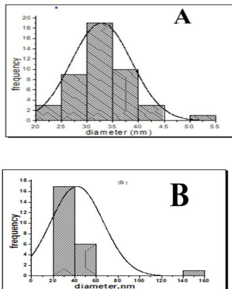
Fig. 7. (A, B) Size distribution histograms of ZnO nanoparticles without and with TEA
