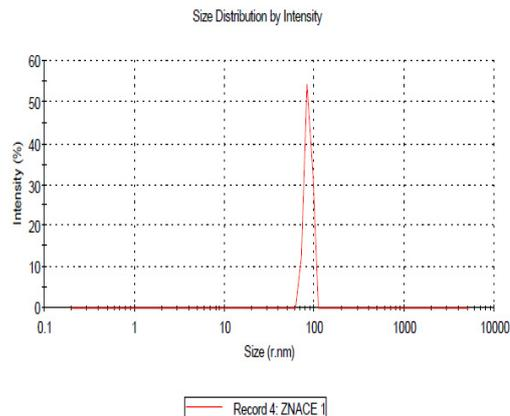
narrow range as shown in figure 4, 5. The particle size of synthesized ZnO powder is about 84.98 nm in with TEA figure (4) While with average size ranging from 250 to 500 nm were observed for without TEA figure (5).
