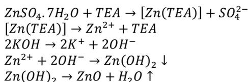
In the Sol-gel case, the amine group of TEA binds to surface ZnO atoms, while the OH groups provide hydrophilicity [20,21]. The TEA molecules passivate the surface and create a steric barrier between neighboring ZnO nanoparticles. A schematic representation of capped ZnO nanoparticles is shown in figure 1.
