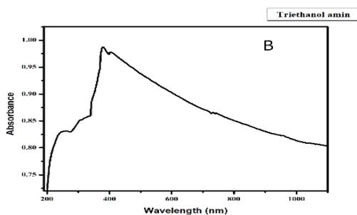
Fig. 8. Electronic absorption of UV-VIS spectra for ZnO nanoparticles A and B.
