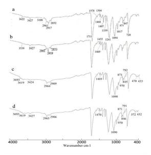
**Figure 4:** FTIR spectra of (a) untreated PET, (b) treated PET/8%NaOH, (c) PET/1% SiO<sub>2</sub>NPs and (d) PFT/1.5% SiO<sub>2</sub>NPs
