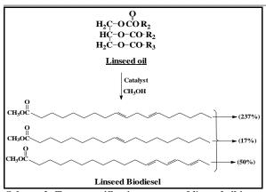
Scheme 2: Transesterification process of *linseed* oil into its corresponding biodiesel.
