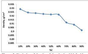
Figure 3: Variation of density of the obtained biofuel by changing the biofuel of castor oil ratio.
