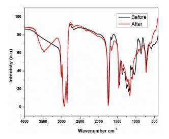
Figure 2: FTIR spectra of linseed oil and biodiesel obtained from linseed oil.
