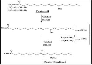
Scheme 3: Transesterification process of *castor* oil into its corresponding biodiesel.
