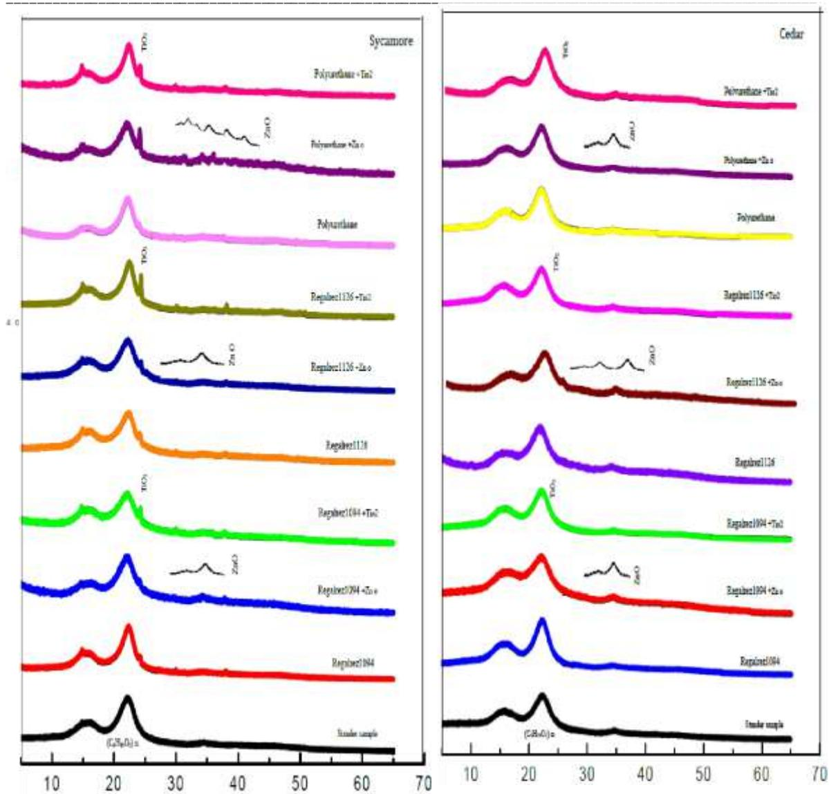
**Fig. 9** X-RD of untreated and treated cedar and sycamore woods by consolidation materials
