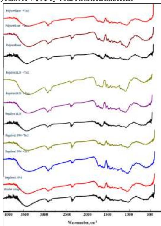
**Fig. 8b** FT-IR spectra of untreated and treated cedar wood by consolidation materials
