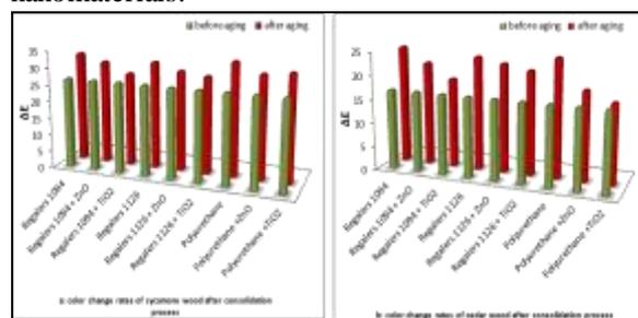
Fig. 5. Difference between color change rates of sycamore and Cedar wood, after consolidation process
