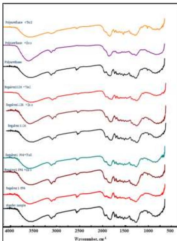
**Fig. 8a** FT-IR spectra of untreated and treated sycamore wood by consolidation materials
