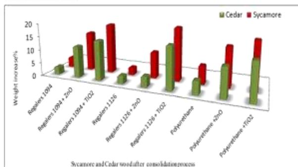
**Fig. 6** The average weight increase in Sycamore and Cedar wood after consolidation process
