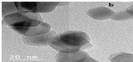
**Fig. 3.** a) XRD  $\text{TiO}_2$ -NPs and b) TEM image of  $\text{TiO}_2$ -NPs
