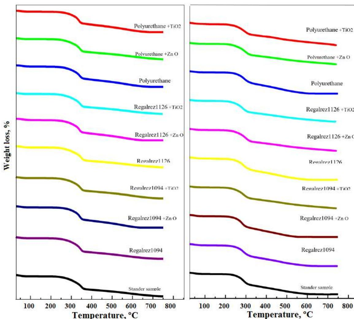
Fig. 10. TGA of untreated and treated cedar and sycamore woods by consolidation materials
