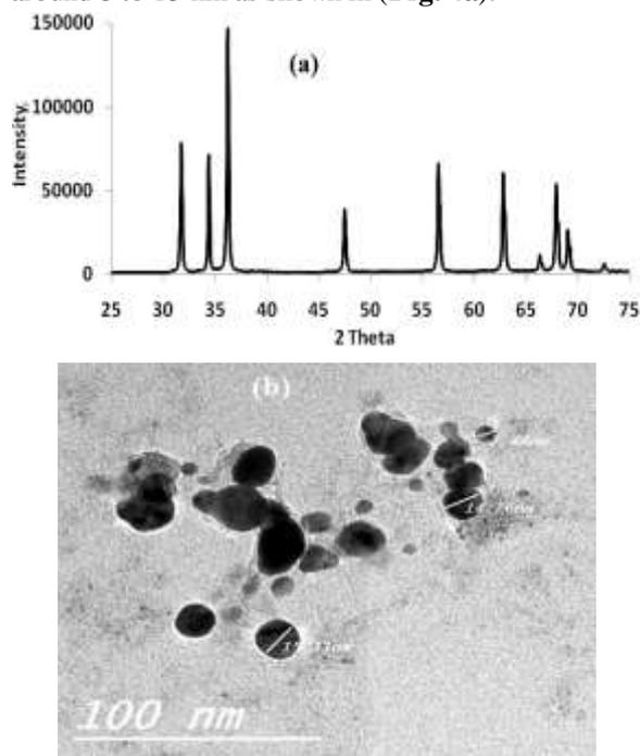
Fig. 4: a) XRD and b) TEM image of ZnO-NPs
