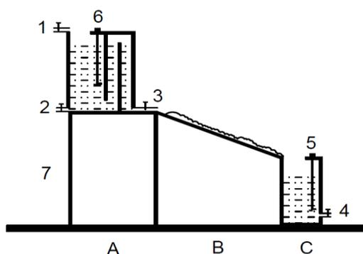
Fig. 1. Schematic diagram of bench-scale engineered system for treatment of drainage wastewater collected from El-Rahawy drain. (A)
