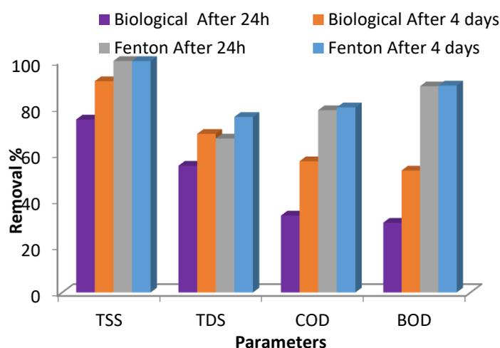
Fig 2. Removal % of TSS, TDS, COD and BOD parameters after biological and Fenton treatment processes
